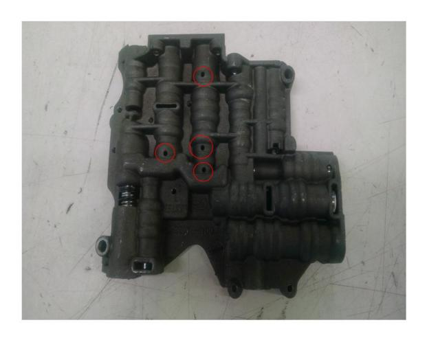
Install .250" plastic check ball in oval slot as shown
