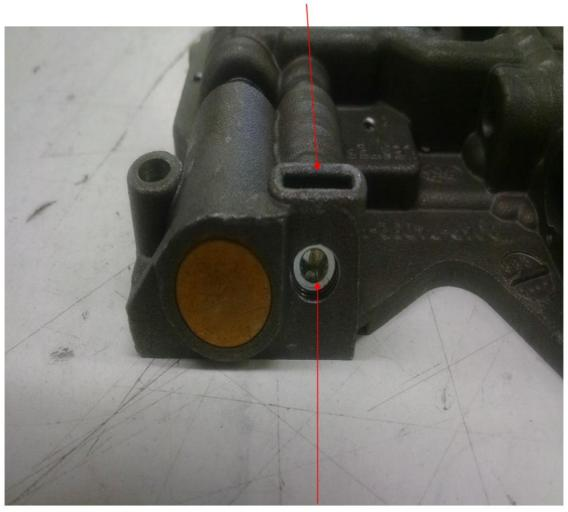
Supplied 1/8" NPT pipe plug installed in bore.
