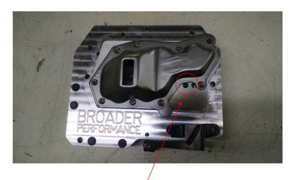
If you are using a different filter than the original style filter shown, be sure the 2 pressure regulator vent holes are not blocked off. This will cause extremely high line pressure that will cause damage to pump etc....
